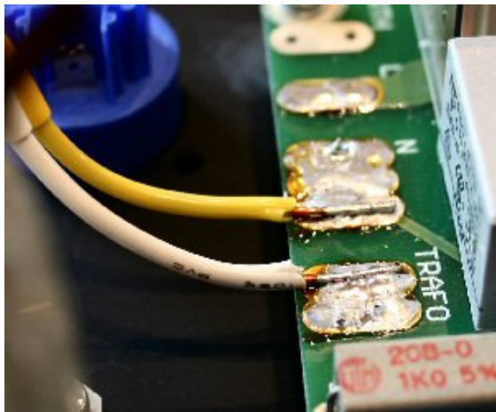
Solder the primary wires of the transformer and secure with cable ties.
