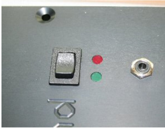
Solder the LEDS when levelled at surface.
