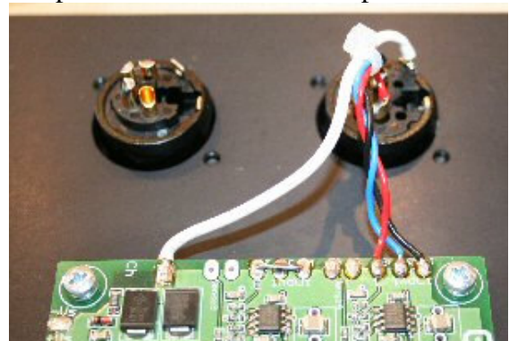
Connect DCN23 ch.A input to XLR 3-pol with 0.2mm wire. Pad/pin1 black, pad/pin2 black, pad/pin3 blue and twist.
