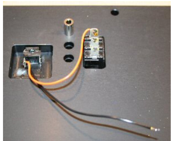
Optional connection of the operation switch with DC control of the AUTO position. Wire connects tip with switch pin closest to edge. Ring of mini jack connects to GND of PSU12SA.
