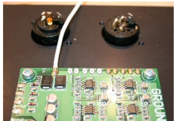
Connect white 0.75mm wire from DCN23 CH pad to NC3FD-L1 chassis pin.
